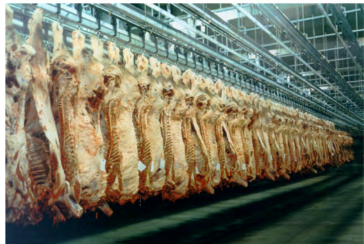
Illustration of loaded walking beam rail showing indexed carcass sides with spray chill system.
