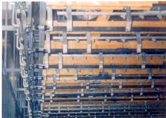
Illustration of walking beam feed-in consisting of head rail, divert switches mounted to wood beams.
