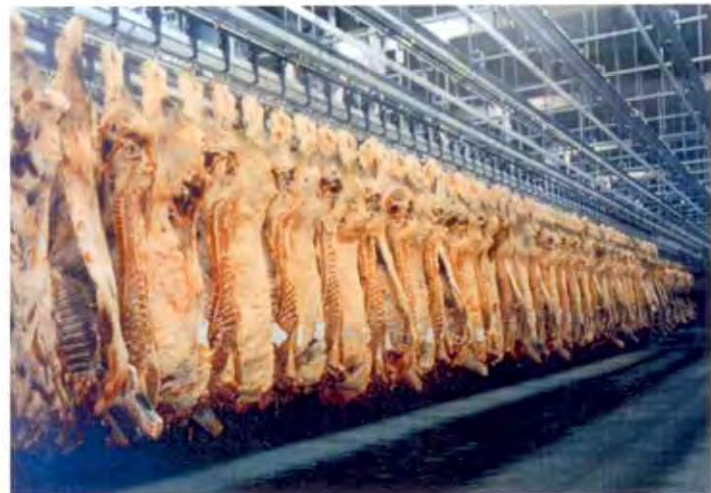
Illustration of loaded walking beam rail showing indexed carcass sides with spray chill system.
